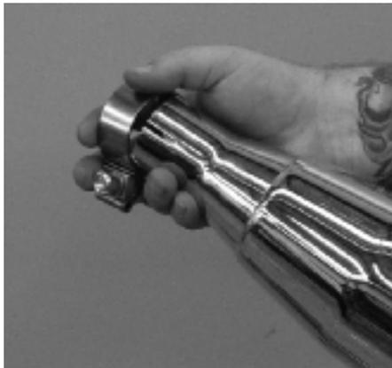
**7** Slip the stock clamp onto the new B-52 muffler. Note the alignment of the clamp. You may want to rotate the pipe to hide the bolt on the clamp.
