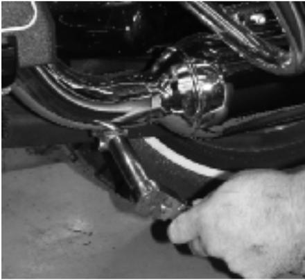
**3** Using a 9/16" socket, Dave removes the clamp that holds the stock muffler to the header pipe. It doesn't matter which muffler you do first.
