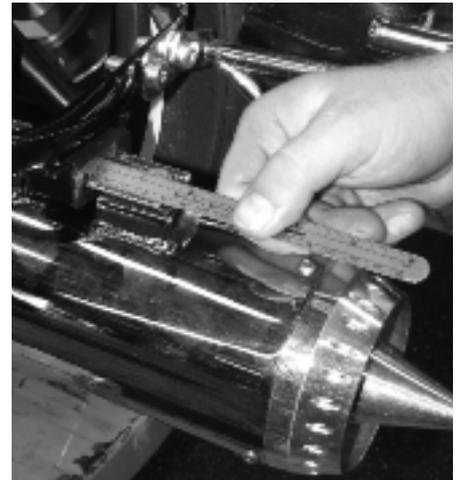
**10** After measuring where each muffler bolts to the bracket to ensure that one is not sticking farther out than the other, fully tighten the muffler bracket bolts.
