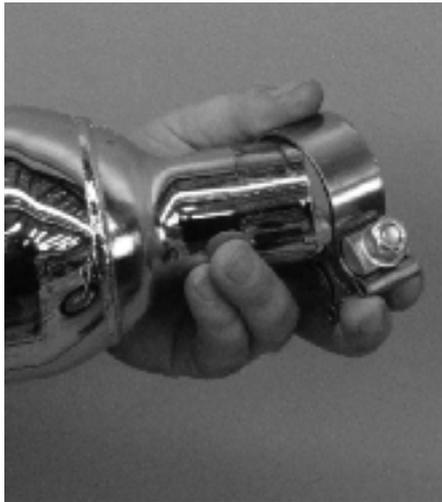
**6** Remove the clamp from the muffler, taking care to inspect it for wear and corrosion. If it's damaged in any way, replace it.
