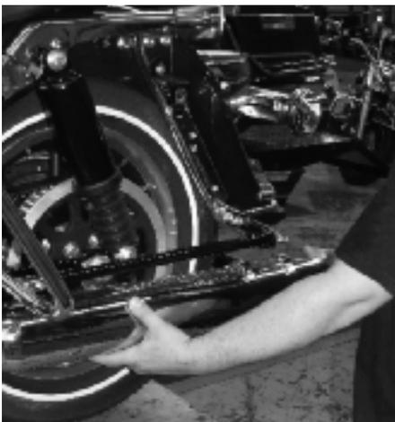
**5** The muffler can now be pulled off its header pipe. You may have to shimmy the muffler from side to side a bit before it comes loose, but it should slip right off.
