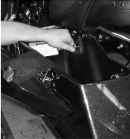
**13** Reinstall the saddlebags using the mounting screws on the inside of each bag.
