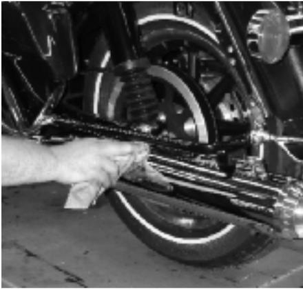
**12** Clean all dirt, oil, and fingerprints off both B-52 mufflers before firing up the motor, or the pipes will be stained permanently.
